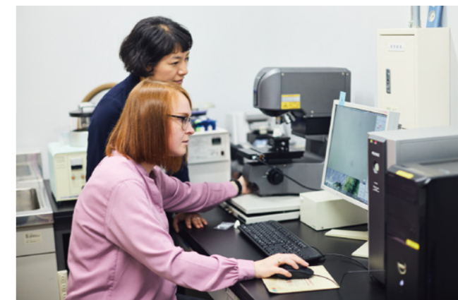
▲Fig. 3. Scanning the wear on tooth surfaces with a confocal laser microscope.
