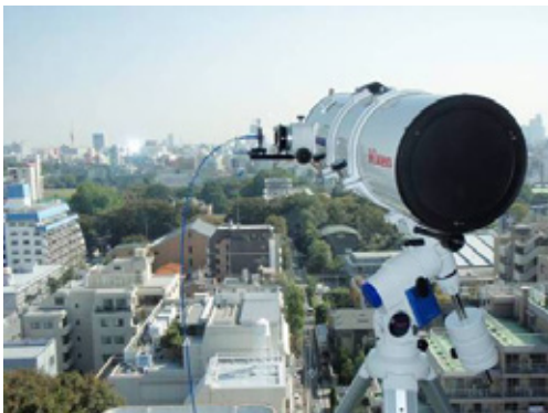
パルス型差分光装置を用いたNO 2 計測 Measurement of atmospheric NO 2 by a pulsed differential absorption optical spectrometer
