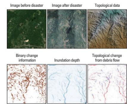
3D change recognition by fusion of simulation and machine learning. Successfully estimating inundation depth during flooding and topographical changes due to debris flow from images before and after the disaster and topological data.
