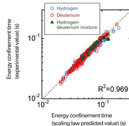
▲Fig. 3. Thermal shielding capacity can be expressed as a time constant, energy confinement time. Multiple regression analysis suggests an accurate prediction model.
