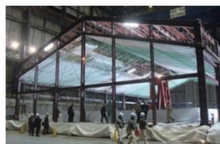
Seismic test of ceiling on shaking table using a real-sized gymnasium
