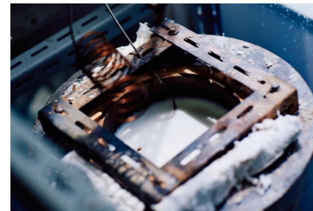
▼ Conducting an experiment using a stainless-steel reactor with a volume of about 10 mL.
