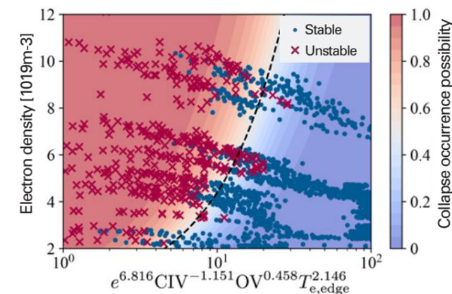
▲Fig. 4. In addition to separating stability and instability for collapse phenomena, distance from the separation border can be quantified as a possibility of occurrence. On the x-axis,  $e$ , CIV, OV, and  $T_{e,edge}$  represent Napier's constant, the line spectrum radiation strength from trivalent carbon ions and tetravalent oxygen ions, and the electron temperature at the plasma edge, respectively.
