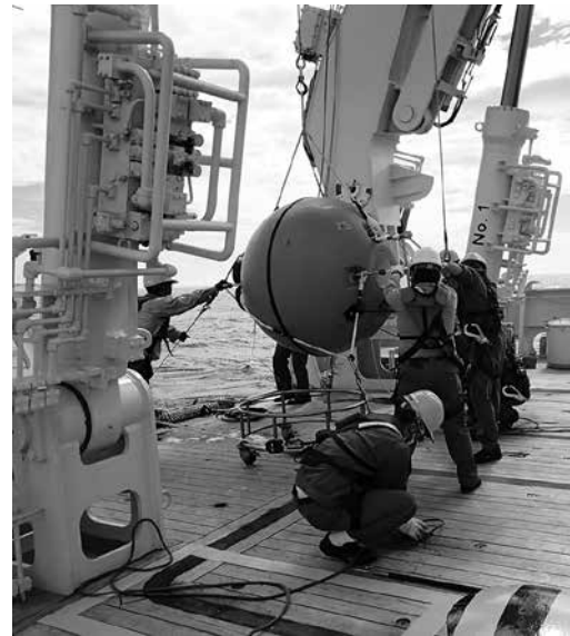
音響多層流速計の設置 Deployment of acoustic current profiler
