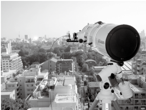
パルス型差分吸収分光装置を用いたNO 2 計測 Measurement of atmospheric NO 2 by a pulsed differential absorption optical spectrometer
