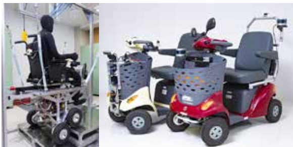
知能化電動車いす (左：階段昇降機能/右：自律移動機能) Intelligent powered wheelchair (Stair climbing function/ autonomous function)
