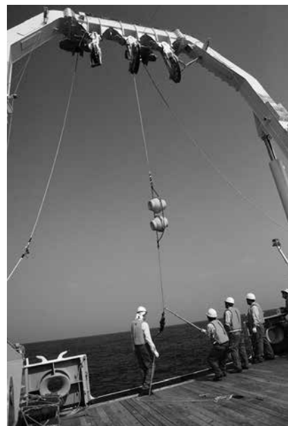
係留系設置作業 Deployment of moored current meter
