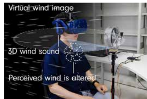
視聴触覚間のクロスモーダル効果を用いた風向知覚操作 Cross-modal Wind Display: Modifying Perceived Directions of Wind Using Visuo-audio-haptic Interaction
