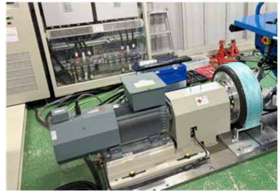
電動モビリティの実走行負荷模擬装置および計測装置 Real-World Driving Load Emulation and Measurement System for Electrified Mobility
