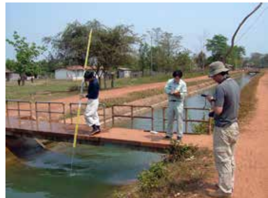
農業用水路における流量・水質観測 Water volume and quality measurement in irrigation canal
